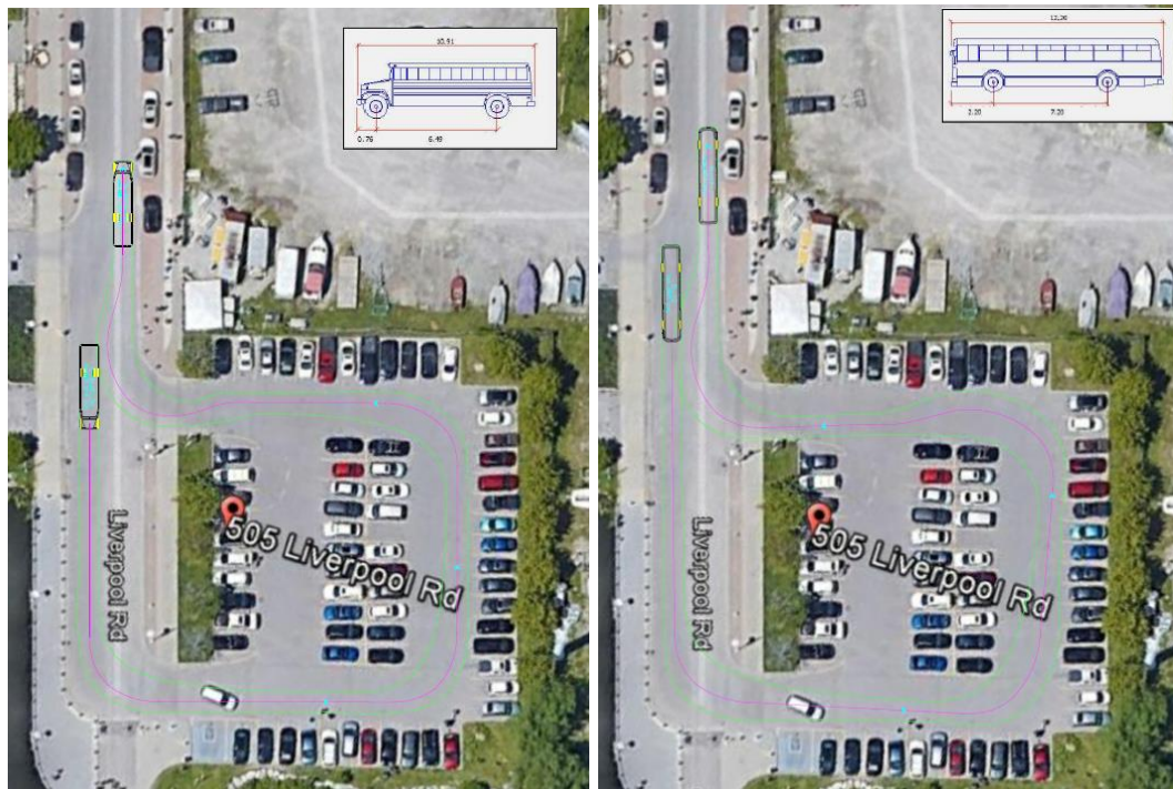
Exhibit 18: Path Swept Analysis of a 36-foot Bus (Left) and 40-foot Bus (Right)
