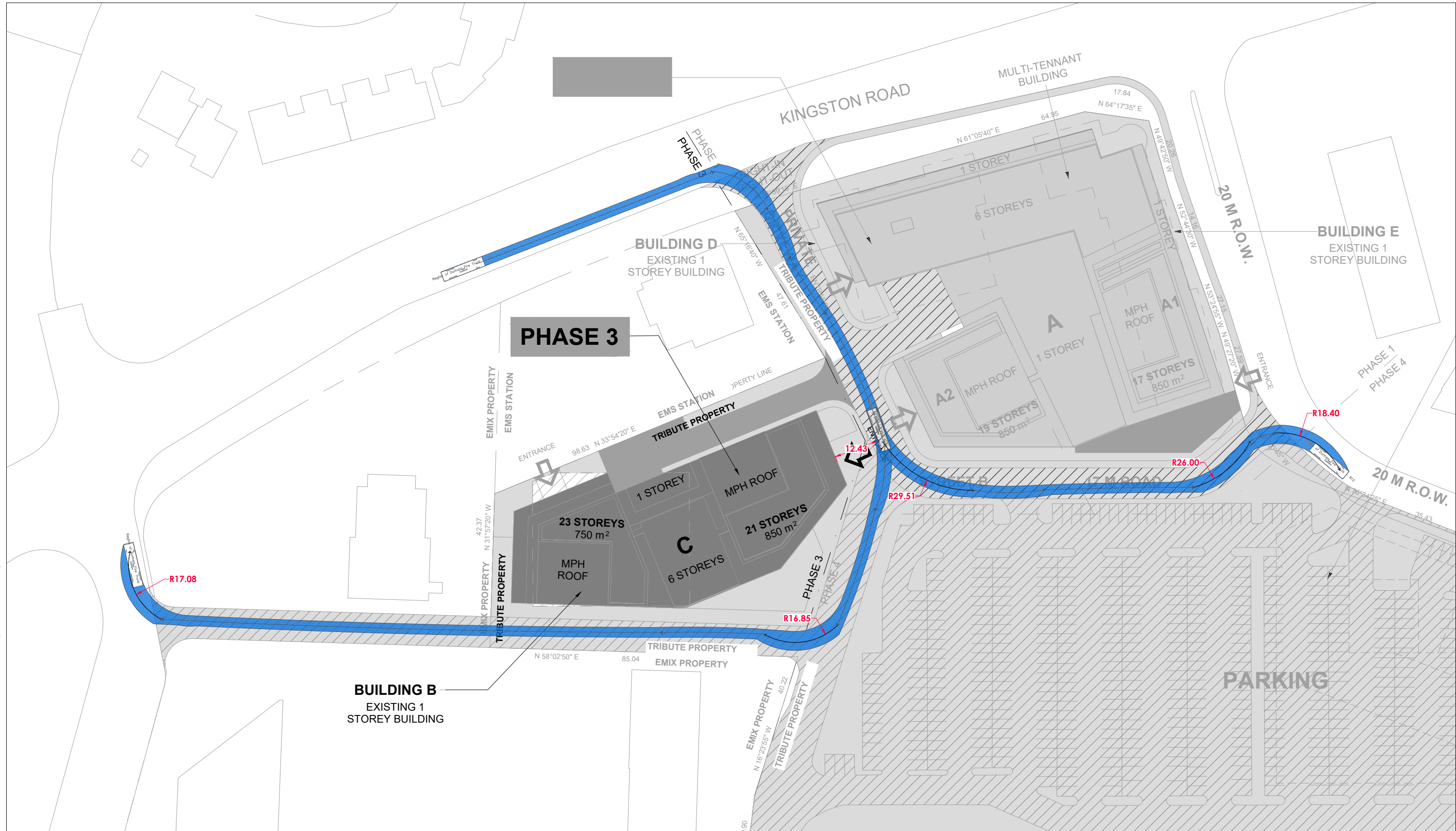
Figure 6-5 Fire Truck Circulation - Phase 3 1105-1163 Kingston Road, Pickering
