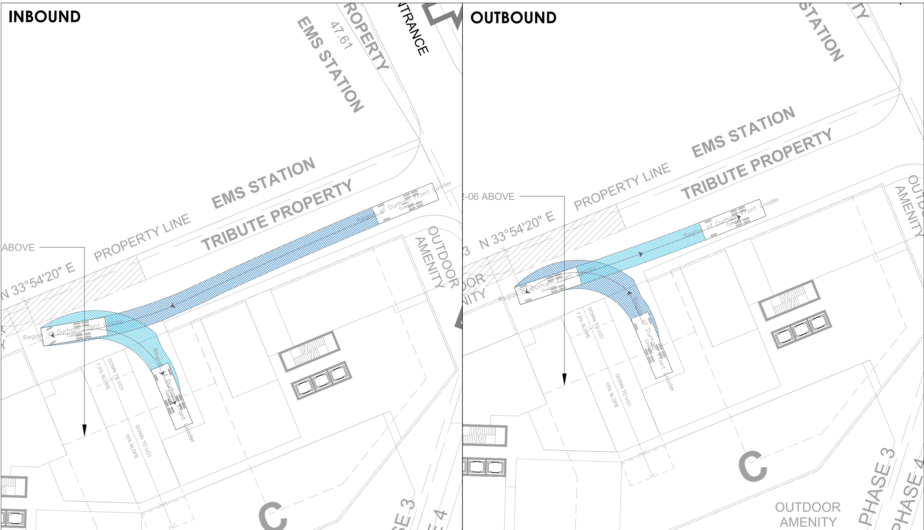
Figure 6-9 Front Loader Garbage Truck Turning Maneuver - Building C 1105-1163 Kingston Road, Pickering
