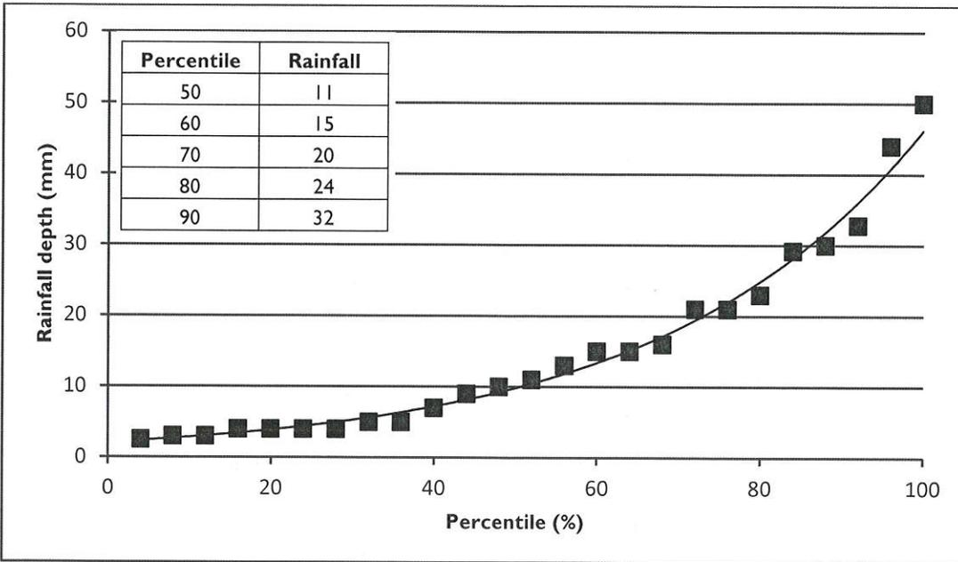
**Figure 2. Rainfall depth frequency curve**
