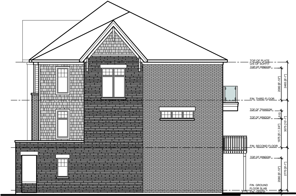
SIDE ELEVATIONS - BUILDING D
