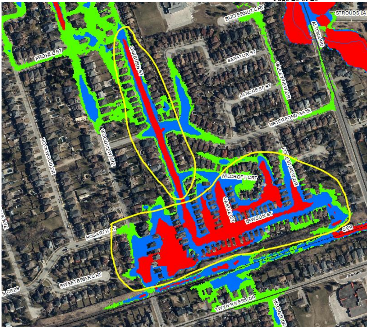
Figure 23 – Distribution of low- moderate- and high-risk flood between Prohill St and CPR railway track.
