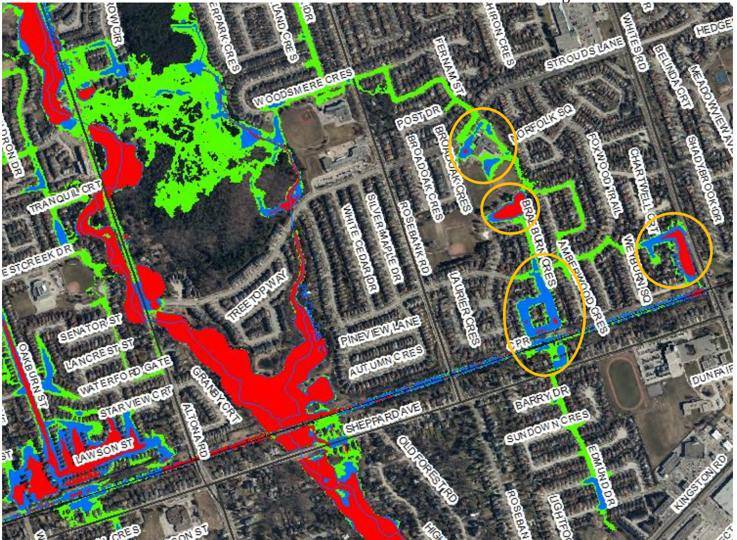
Figure 25 – Distribution of low- moderate- and high-risk flood in Highbush P.S. and along Gardenvue Sq./Weyburn Sq. area.
