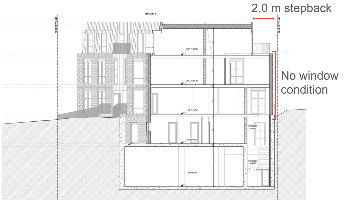
Block 3 - rear building stepback at Liverpool frontage and elevation consideration for transitional design
